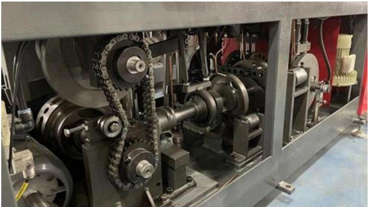
1. The whole **Middle Speed Paper Cup Machine** adopts automatic oil lubrication system( oil circulation system is including oil motor,filter, copper pipe )which makes all gear moving parts working at high speed much more smoothly and greatly Improve the service life of spare parts.
